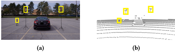
Figure 13: The visualizations of a real-world adversarial example after shifting the adversarial objects. (a) The new locations of adversarial objects after shifting. (b) The segmentation result after shifting.
