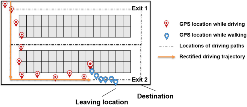
Fig. 4. An example of trajectory and destination extraction.
