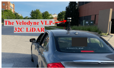
Figure 9: The LiDAR perception testbed with a Velodyne VLP-32C LiDAR.
