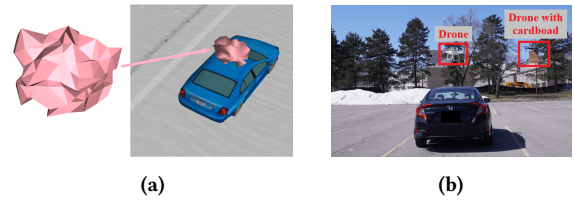
Figure 1: Two examples of object-based LiDAR attacks. (a) The attack using an object with a specific shape [45]. (b) The attack using objects with arbitrary shapes [60].
