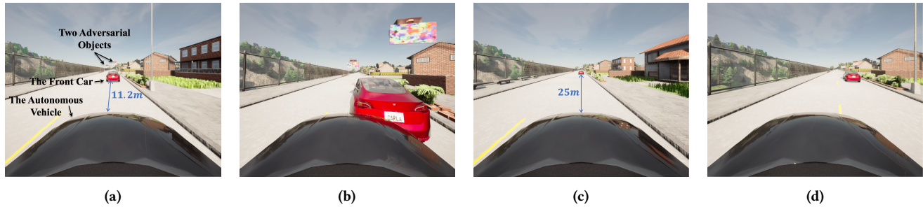
Figure 8: Impact of our defense on autonomous vehicle behavior. (a) The first LiDAR frame in which the car in front is detected when there is no defense. (b) The autonomous vehicle collides with the front car when there is no defense. (c) The first LiDAR frame after the attack is detected and verified using our defense. (d) The autonomous vehicle successfully changes lanes after the attack detection using our defense.
